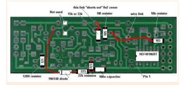
Refer to the placement diagram for the position of each component. The resistors are identified by either 3 digits or 4 digits.
