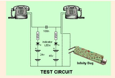
Connect the Bug to the test circuit shown above and pick up the left-hand phone.
