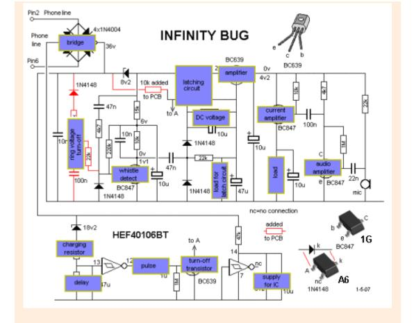
The Infinity Bug connects across the phone line and takes very little current as most of the circuit is not active when in the "waiting" state.
